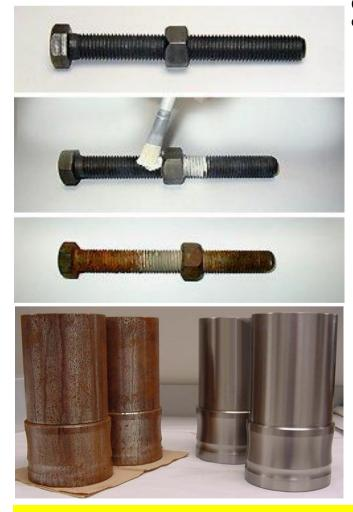
**Vorta RPO** can be applied by dipping, brushing, spraying or swabbing.
